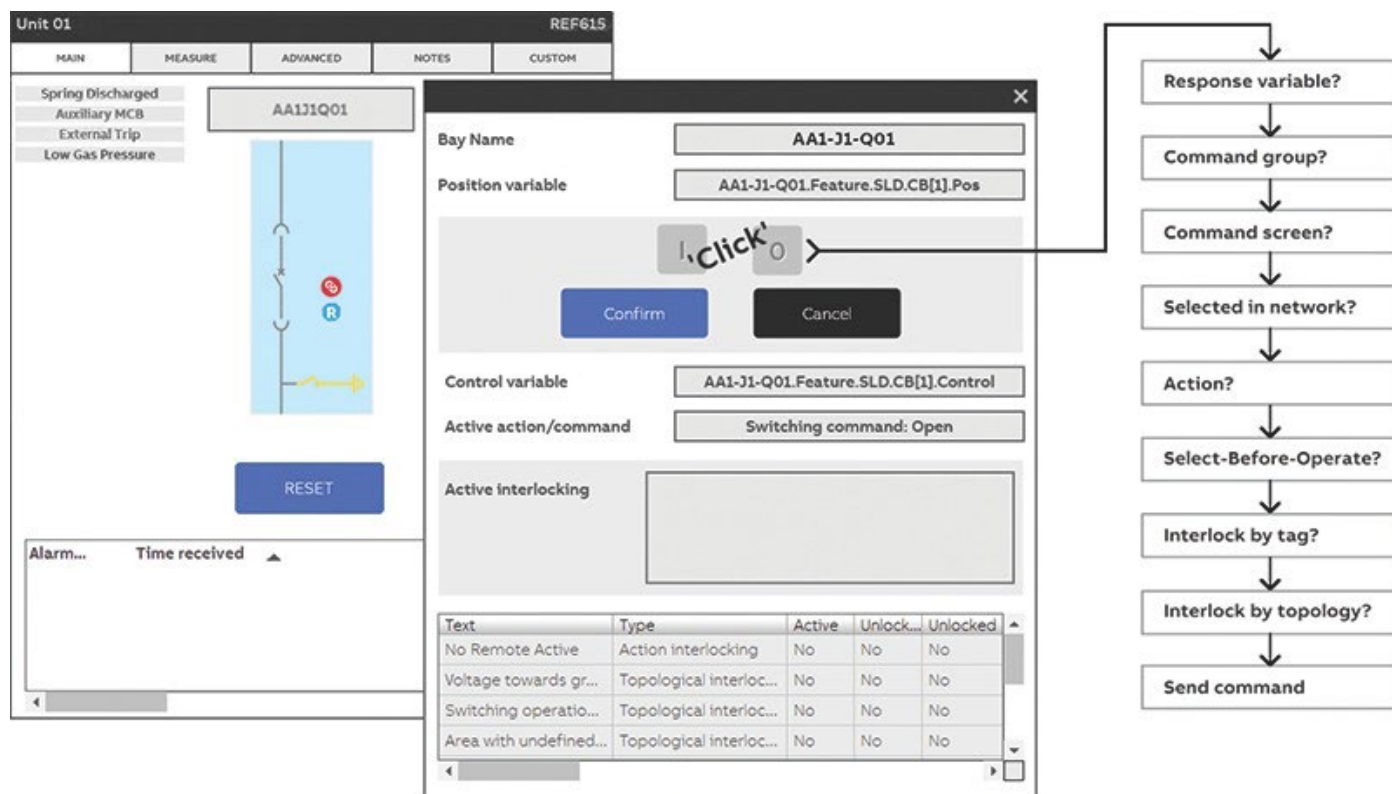
Figure 16. Secure command processing (interlocking and topology check)
